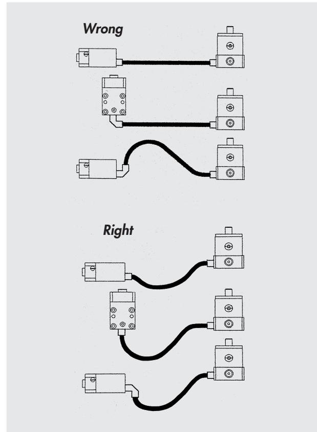
**Required position of H1 as compared to H2** See above for proper positioning of the H1 Pump.
