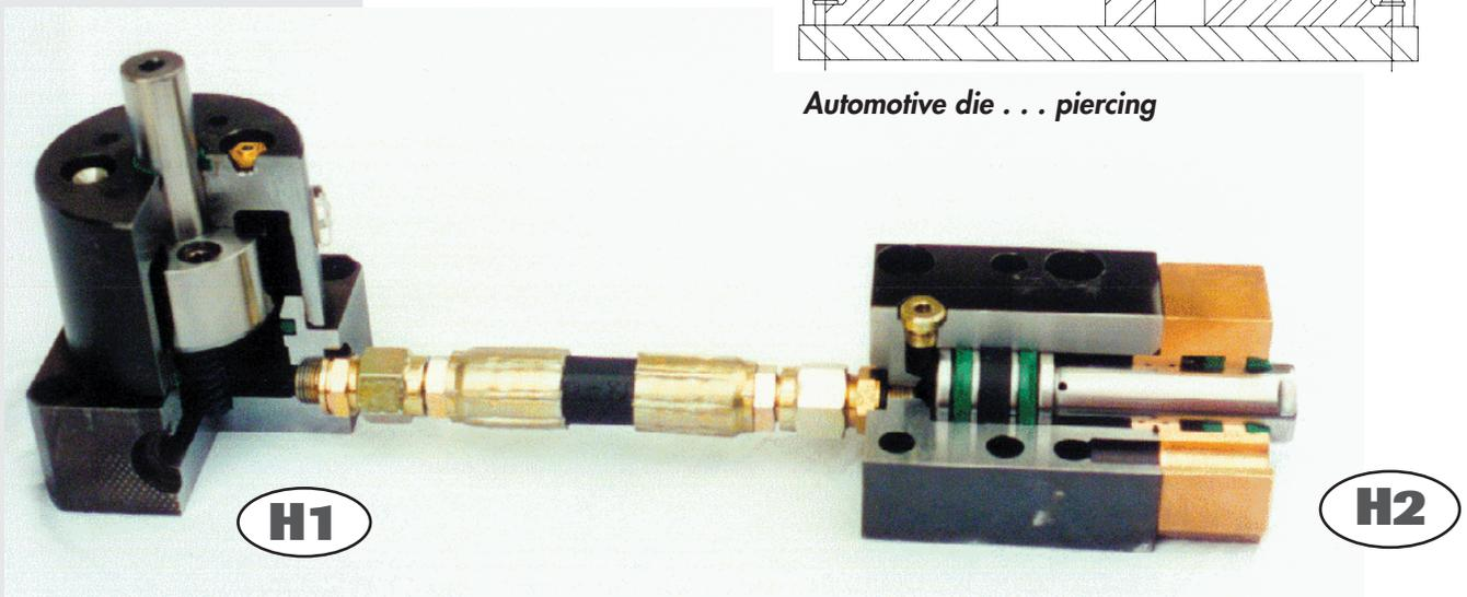
**NOTE:** **HYDROCAM®**'s unique design eliminates the thrusting force of the ram/slide from the cam station, allowing the use of standard L-GIBS to position and guide the station. Providing a guidance system for a **HYDROCAM®** driven cam station is the responsibility of the customer. Neither, the H2 unit's piston rod, nor its front mounting plate assembly is designed to provide cam station guidance. Contact your representative for application support.
