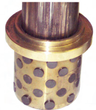
Actual test photo of a graphite plug bushing. See how the plugs extrude.
