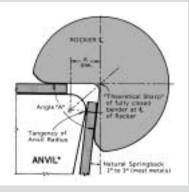
\*NOTE: The back taper relief ground on the anvil is to allow for the overbend required without pinching the material at full closure. (85° minimum anvil angle suggested for all 90° bends). Always grind 2° to 3° more back taper on anvil than the rocker's angle "A" being used.
