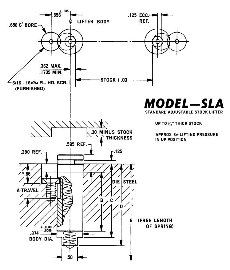
\*DEPTH IS FOR STANDARD TRAVEL INCREMENTS OF 1/4 INCH INCREASE DEPTH TO DECREASE TRAVEL BETWEEN STANDARD SIZES
